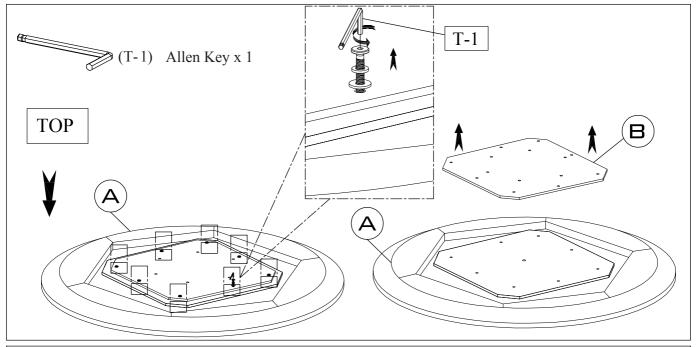
Using a second person to assist you, carefully place the Table Top (A) upside down onto a padded, non-marring surface. Use provided Allen key (T-1) to remove the Allen Bolts (H-2), Spring Washers (H-3) and Flat Washers (H-4). Save all hardware for the following steps. Place Base Top Plate (B) aside.
