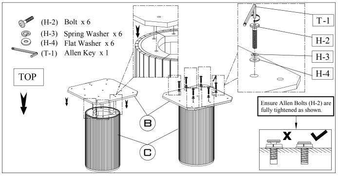
Using a second person to assist you, carefully place the Table Base (C) right side up. Position the Base Top Plate (B) so that the through holes line up with the threaded inserts in the Table Base (C). First, insert and engage the Allen Bolts (H-2), Spring Washers (H-3) and Flat Washers (H-4) using the provided Allen Key (T-1), stacking the hardware in the order as shown. Once all have been engaged, fully tighten. DO NOT OVER TIGHTEN
