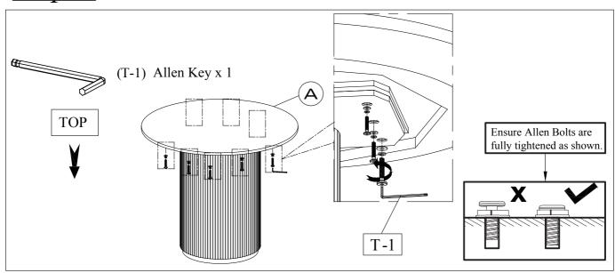
Align the threaded inserts in the Table Top (A) with the through holes in the Base Top Plate (B). Secure by first engaging all Allen Bolts (H-2), Spring Washer (H-3) and Flat Washer (H-4) first by hand, then fully tighten using the provided Allen Key (T-1), stacking the hardware in the order as shown. DO NOT OVER TIGHTEN.
