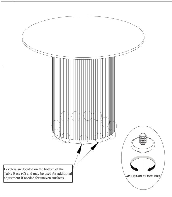
Assembly is now complete and the product is ready for use. Adjustable levelers are located on the bottom of Table Base (C) and may be adjusted by turning outwards, counter-clockwise to help account for uneven surfaces. NOTE: Hardware may loosen over time. Periodically check that all connections remain tight and adjust as needed.
