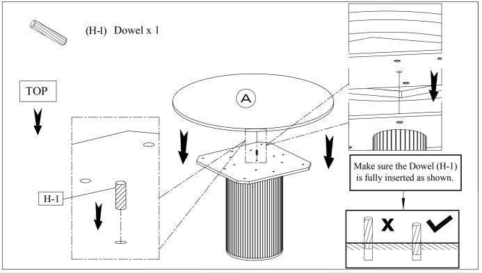
Insert the Dowel (H-1) into the center hole in the previously installed Base Top Plate (B). Ensure that it is fully seated. Using a second person to assist you, carefully lower the Table Top (A) down onto the assembly so that the Dowel (H-1) inserts into the receiving holes underneath the Table Top (A).
